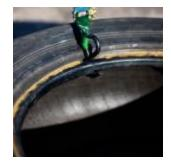
Drill a hole in the tire. Put the hook of the truck strap through the hole. *If you are using a rope:* Get an eye bolt, two hole bolts, and two washers. Put the eye bolt through the hole bolt and washer on either side of the tire. Secure the rope to the eye bolt.
